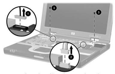
Disconnecting the Display Cables and Removing the Display Assembly Screws
